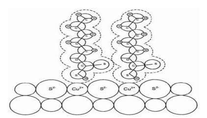
Sketch of attachment of amy! xanthate ions to covellite. There is a hydrogen atom bidden behind each carbon of the hydrocarbon chain
