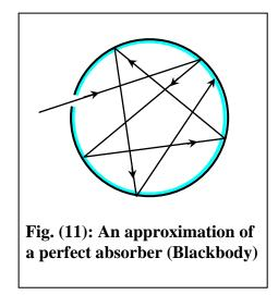
through the hole, so that after many internal reflections nearly all the radiation is absorbed and the body approximates a blackbody.
