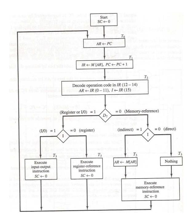
C- Direct Address Instruction has its operand address specified directly in the instruction, but the Indirect Address Instruction has the address of the operand's address, i.e. not directly the address of the operand.
